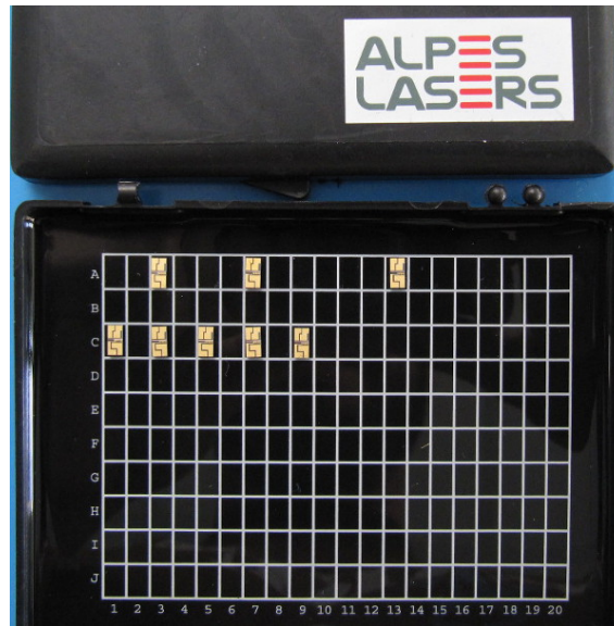
Figure 3.2.: AN and HP-GS mounted ALPES LASERS QCL gel pack.
