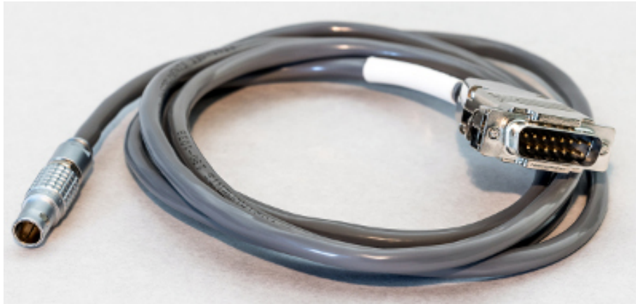
Figure 5.18.: C-TC-3-LLH cable connecting the LLH housing to the TC-3 temperature controller.
